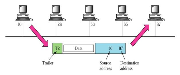
Most local area networks use a 48-bit (6 bytes) physical address written as 12 hexadecimal digits, with every 2 bytes separated by a hyphen as shown: 07-01-02-01-2C-4B
