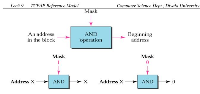
The network address is the beginning address of each block. It can be found by applying the default mask to any of the addresses in the block (including itself). It retains the netid of the block and sets the hostid to zero.
