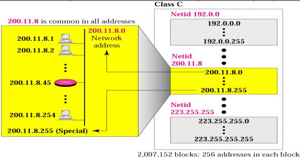
The number of addresses in a class C block is smaller than the needs of most organizations. Class D addresses are used for multicasting; there is only one block in this class. Class E addresses are reserved for special purposes; most of the block is wasted.
